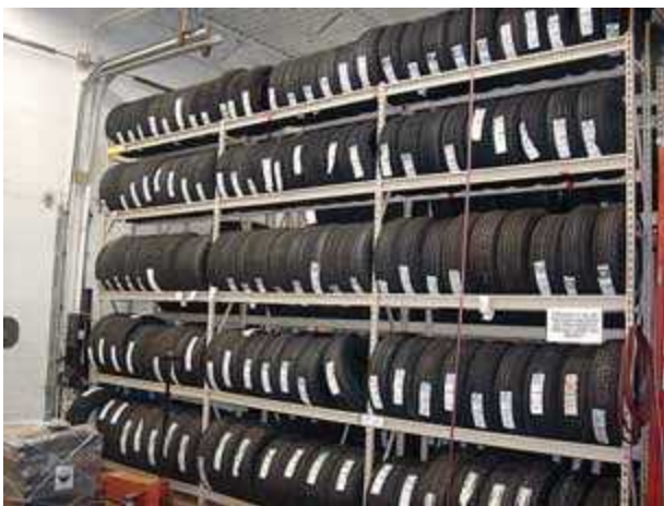
On-tread tire storage on racks.
