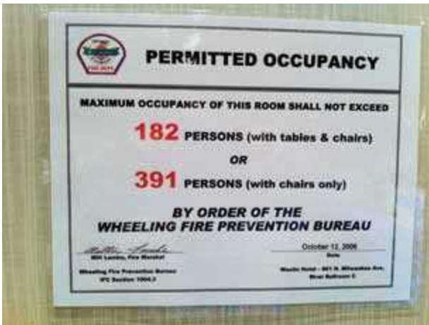
Dual occupant load postings indicative of two common uses of a space.
