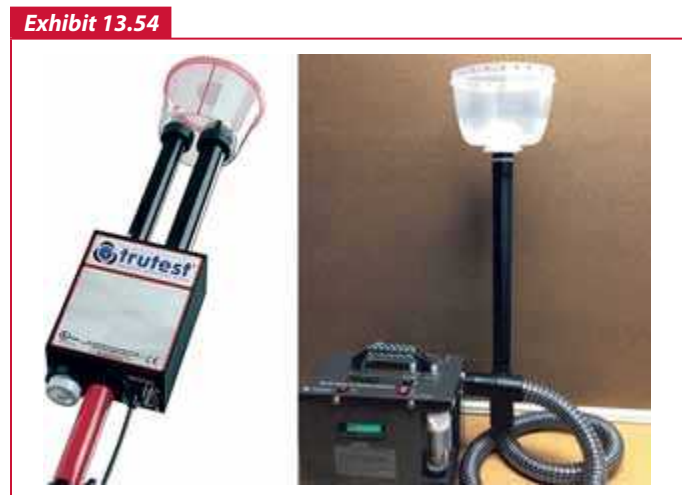
Test Equipment. (Left) Smoke Detector Sensitivity Tester (Courtesy of SDI, LLC, Neptune, NJ); (Right) A Calibrated Smoke Detector Sensitivity Test Instrument. (Source: Gemini Scientific, Sunnyvale, CA)
