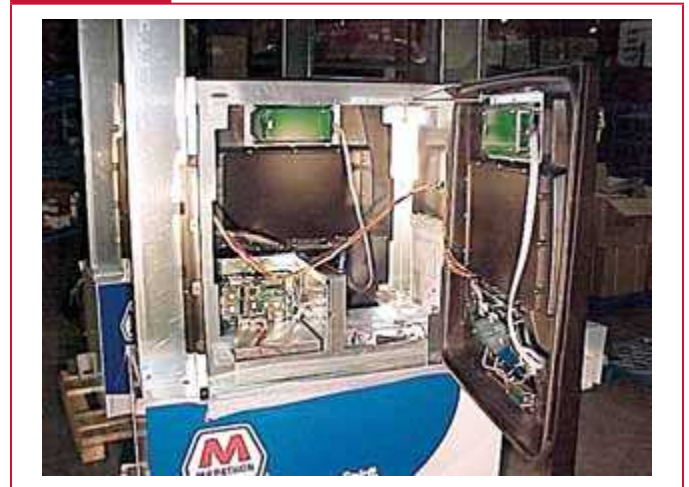
Interior view of electronics cabinet of the fuel dispenser shown in Exhibit 42.11. (Courtesy of Bennett Pump Company, Spring Lake, MI)
