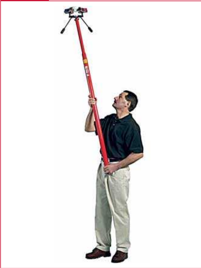
Removal Tool Used to Remove Detectors on High Ceilings. (Courtesy of SDI, LLC., Neptune, NJ)
