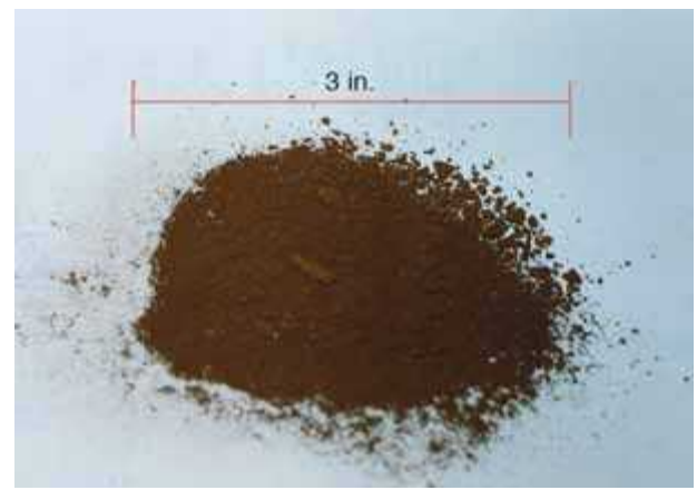
Rust and scale removed from dry pipe system.
