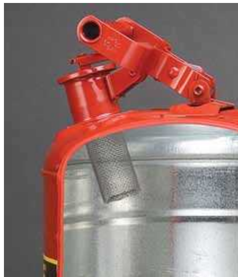
Internal view of safety can showing flame arrester below spout. (Courtesy of Justrite Manufacturing Co.)
