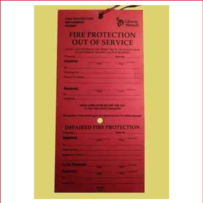
Emergency impairment notice. (Courtesy of Liberty Mutual Commercial Markets)
