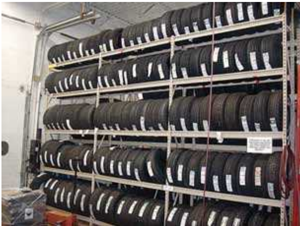
On-Tread Tire Storage on Racks.
