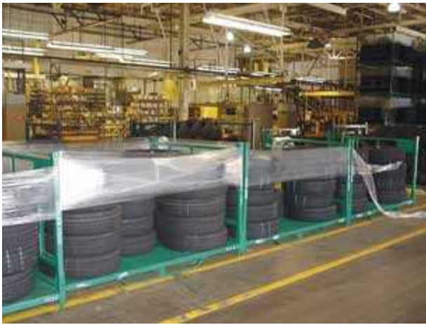
On-side tire storage on portable racks. (Courtesy of Ford Motor Company)
