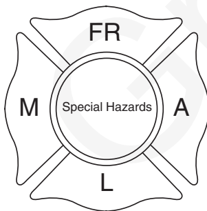
FIGURE D.1.2.3 Sample Sign for Fire Fighter Safety Building Marking System. [1:Figure E.1.2.3]
