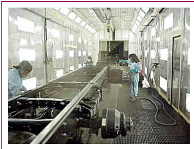
EXHIBIT 516.1 An enclosed paint spray room.
