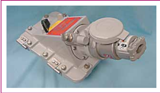
EXHIBIT 501.21 A receptacle and attachment plug of the explosionproof type with an interlocking switch. The switch must be in the "off" position before the attachment plug can be inserted or removed. (Courtesy of Appleton®, Emerson Electric Co.)
