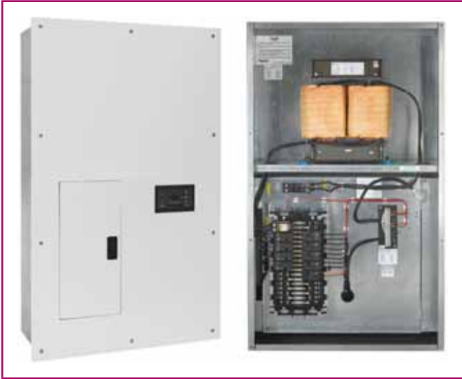
EXHIBIT 517.7 An example of a hospital isolated power system panel with built-in isolation transformer, line isolation monitor, load center, and grounded busbar. (Courtesy of Schneider Electric)
