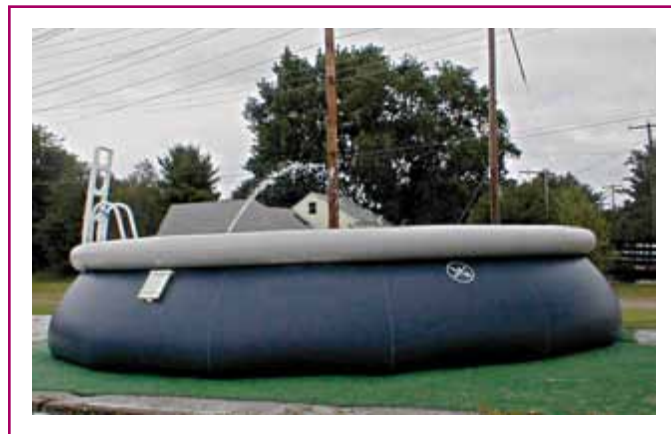
EXHIBIT 680.10 Example of an inflatable swimming pool subject to the requirements in Parts I and III of Article 680.
