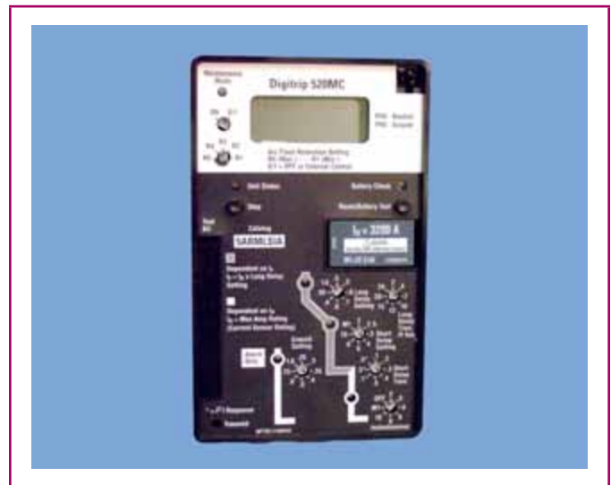
EXHIBIT 240.16 An electronic trip unit for a circuit breaker that has its instantaneous setting set to “off” and that incorporates an energy-reducing maintenance setting. (Courtesy of Eaton)
