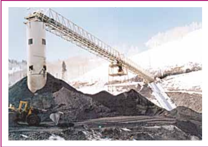
EXHIBIT 500.2 A coal-handling operation classified as both a Class I and a Class II location. (Courtesy of Noel Williams)
