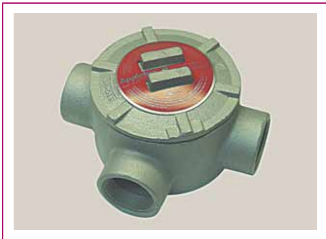
EXHIBIT 502.1 Junction box with threaded hubs, suitable for use in Class II, Group E hazardous atmospheres. (Courtesy of Appleton®, Emerson Electric Co.)
