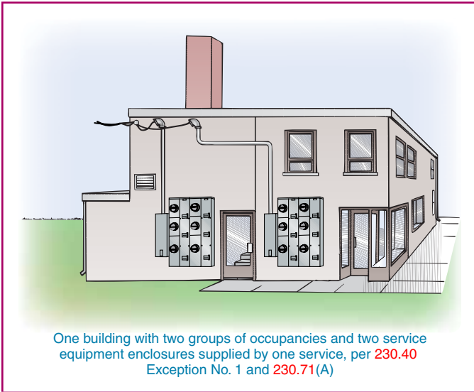
EXHIBIT 230.3 One service drop or one set of overhead service conductors supplying two service equipment enclosures installed at separate locations.
