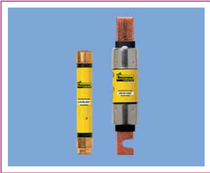
EXHIBIT 240.1 Class R current-limiting fuses with rejection feature to prohibit the installation of non-current-limiting fuses. (Courtesy of Eaton, Bussmann Division)
