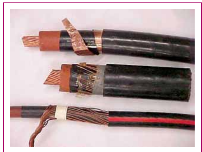
EXHIBIT 250.53 Three examples of single-conductor shielded cable, each having a different type of shielding. (Courtesy of Chuck Mello)
