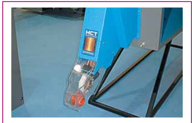
EXHIBIT 665.2 A solid-state induction welding machine. (Courtesy of Thermatool Corp.)
