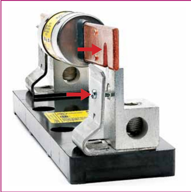
EXHIBIT 240.13 A fuse block rejection pin and notch in the fuse blade (red arrows) ensure that circuit protection is provided by fuses with a specific level of overcurrent protection. (Courtesy of Eaton, Bussmann Division)
