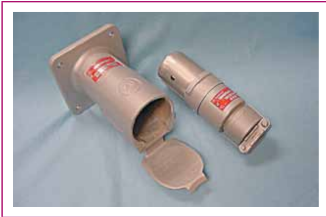
EXHIBIT 501.22 A 4-pole (delayed action) explosionproof receptacle and attachment plug suitable for use without a switch. (Courtesy of Appleton®, Emerson Electric Co.)
