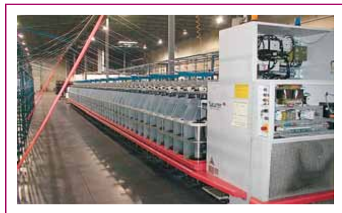
EXHIBIT 670.1 Thread-spooling machine used in the textile industry. (Courtesy of the International Association of Electrical Inspectors)
