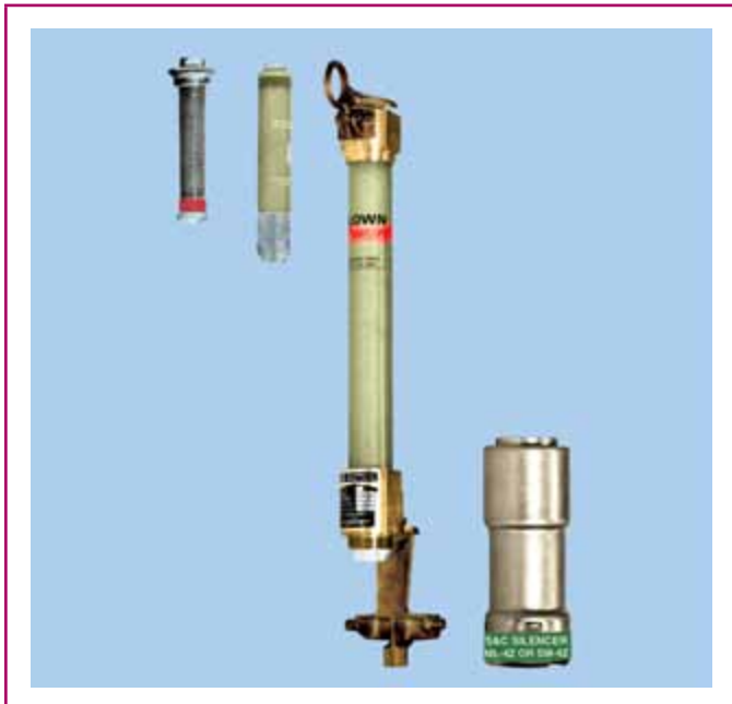
EXHIBIT 490.2 Components of the indoor solid-material (SM) power fuseholder (boric-acid arc-extinguishing type) with a 14.4-kilovolt, 400E-ampere maximum, 40,000-ampere rms asymmetrical interrupting rating. (Courtesy of S&C Electric Co.)
