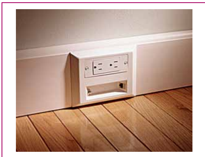
EXHIBIT 388.1 An example of a surface nonmetallic raceway, resembling base molding, that supplies a receptacle outlet on the top and CATV and communications on the bottom. (Courtesy of Legrand/Wiremold®)
