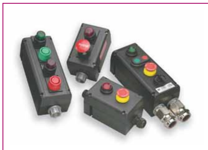
EXHIBIT 505.1 Typical control stations with the combination of flameproof and increased safety types of protection suitable for use in Class I, Zone 1 areas. (Courtesy of Eaton, Crouse-Hinds Division)
