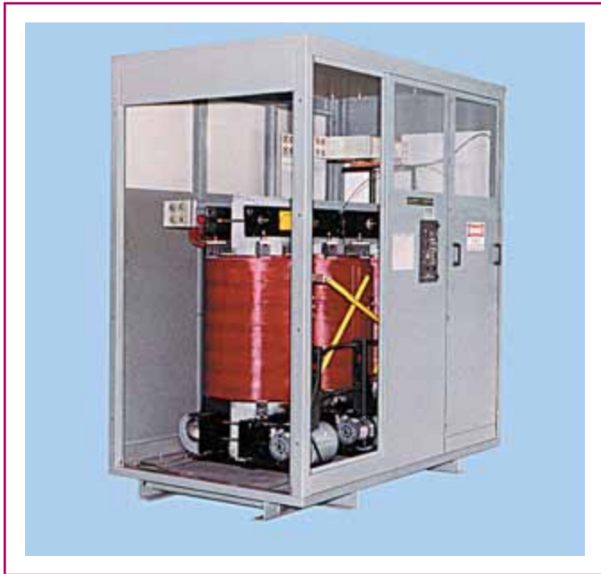
EXHIBIT 450.12 A dry-type transformer with a core and coil design rated at 1000 kilovolt-amperes, 13,800 volts to 480 volts, 3-phase, 60 hertz. Note cooling fans beneath each winding. (Courtesy of Schneider Electric)
