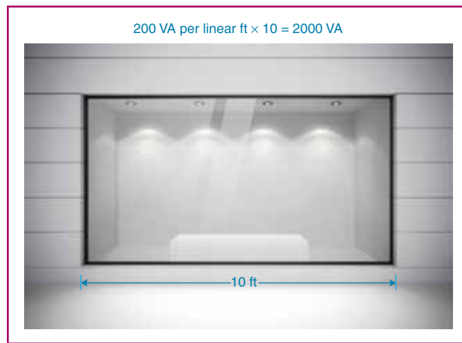
EXHIBIT 220.1 An example of the volt-ampere per linear-foot load calculation for branch circuits serving a show window. (iStockPhoto)
