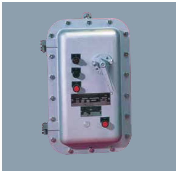
EXHIBIT 501.15 A magnetic motor starter for use in a Class I, Group D location. Note the number of securing bolts and the width of the flange. (Courtesy of O-Z/Gedney, Emerson Electric Co.)
