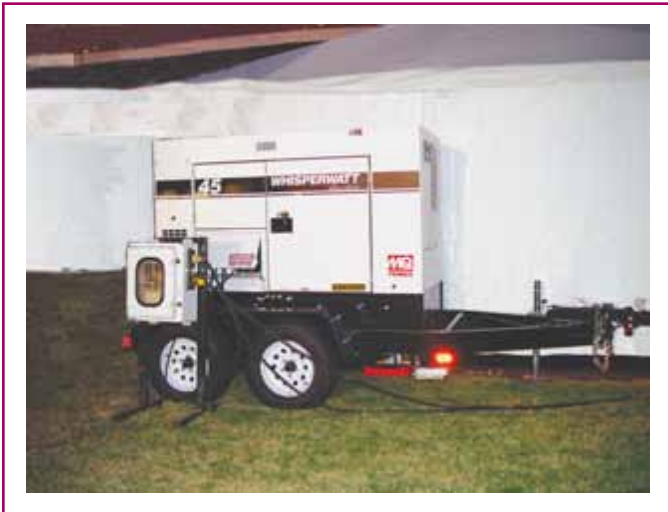
EXHIBIT 702.1 A trailer- (vehicle-) mounted portable generator. (Courtesy of the International Association of Electrical Inspectors)
