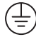
FPN Figure 250.126 One Example of a Symbol Used to Identify the Grounding Termination Point for an Equipment Grounding Conductor.
