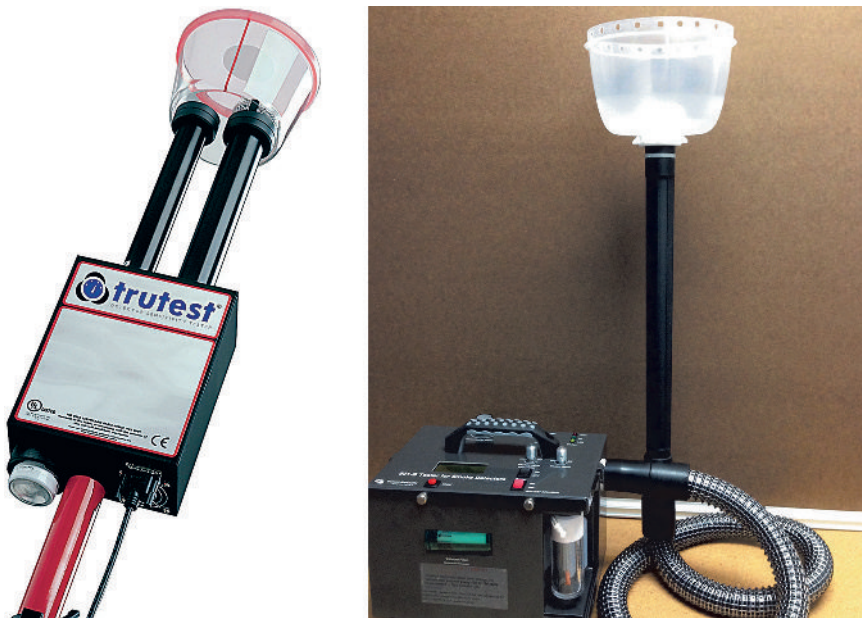
Test Equipment. (Left) Smoke Detector Sensitivity Tester (Courtesy of SDi, LLC, Neptune, NJ); (Right) A Calibrated Smoke Detector Sensitivity Test Instrument. (Source: Gemini Scientific, Sunnyvale, CA)
