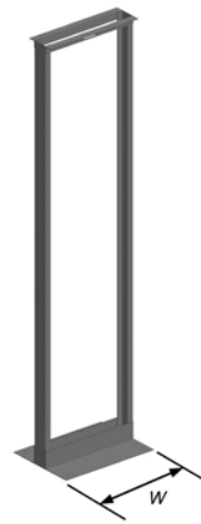
TWO-POST OPEN RACK (Footprint = W \times Datacom Equipment Depth)
