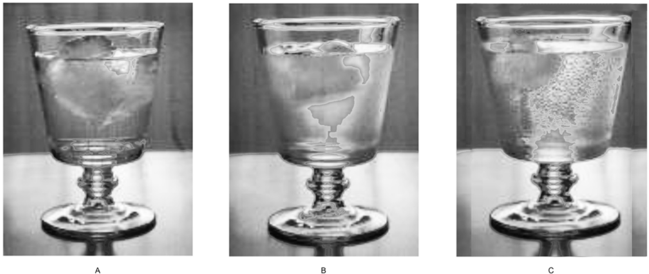
Fig. 2 Stages of Moisture Condensation on Glass (Courtesy Desert-Aire Corp)
