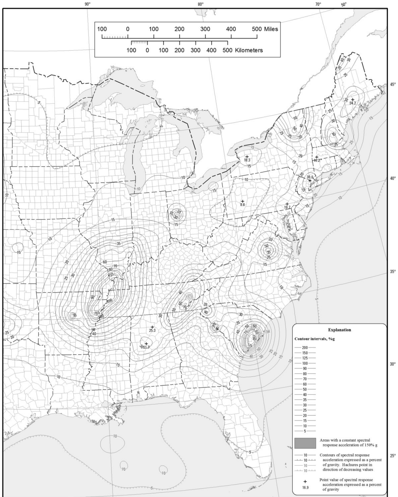
FIGURE 1613.2.1(1)—continued RISK-TARGETED MAXIMUM CONSIDERED EARTHQUAKE ( MCE_R ) GROUND MOTION RESPONSE ACCELERATIONS FOR THE CONTERMINOUS UNITED STATES OF 0.2-SECOND SPECTRAL RESPONSE ACCELERATION (5% OF CRITICAL DAMPING)
