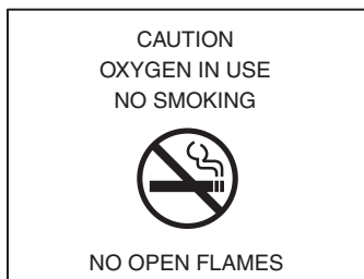
▲ FIGURE A.11.5.3.2 Suggested Minimum Text for Precautionary Signs.
