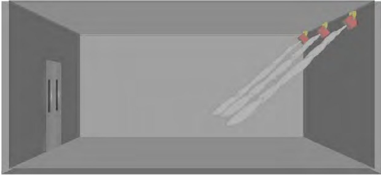
Figure 11.3 – WRONG FirePro Xtinguish condensed aerosol arrangement
