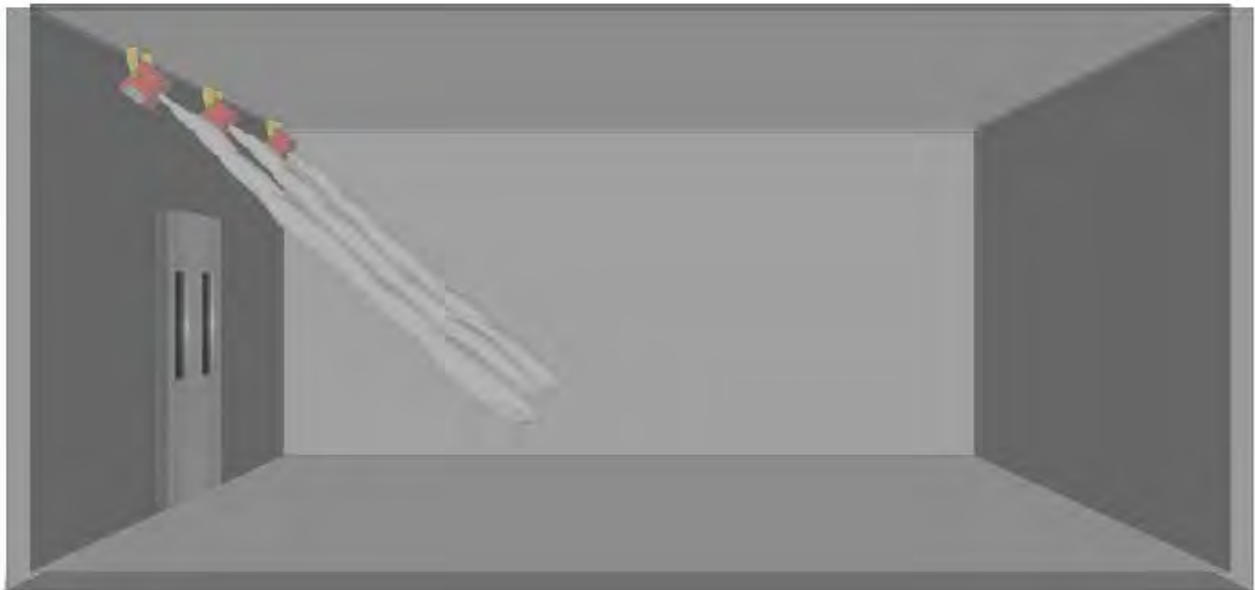
Figure 11.4 – Allowed FirePro Xtinguish condensed aerosol arrangement
